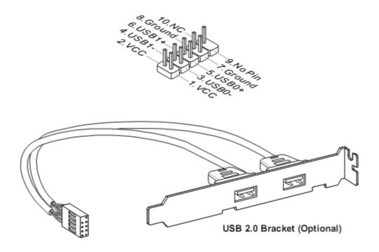
Note that the pins of VCC and GND must be connected correctly to avoid possible damage.
